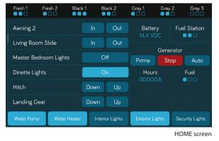
iN-Command<sup>®</sup> is equipped with a Travel Lock Out feature to ensure certain system functions are unavailable during transit. When the Brake signal or the Tow signal is activated, iN-Command<sup>®</sup> will lock down all motorized functions. The DC and mobile devices will display "Travel Lock Out" and affected buttons will display "Disabled". To turn the Travel Lock Out off, the "Unlock" button on the DC inside of the RV must be pressed.
